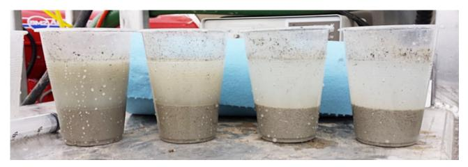
In the above photo, you can see that the solids have settled to the bottom of the container. This is the result you should obtain after 15-20 seconds.
