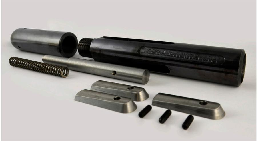
3. Lower the rod string a few inches to retract the 3 locking wedges. Refer to your mark on the rods. Keys will retract and disengage the fishing tool from the rods.
