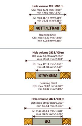
Reaming Shell OD: max 60,07 mm/2.365" min 59,82 mm/2.355"
