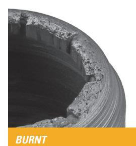
Matrix has completely melted, waterways are closed.
