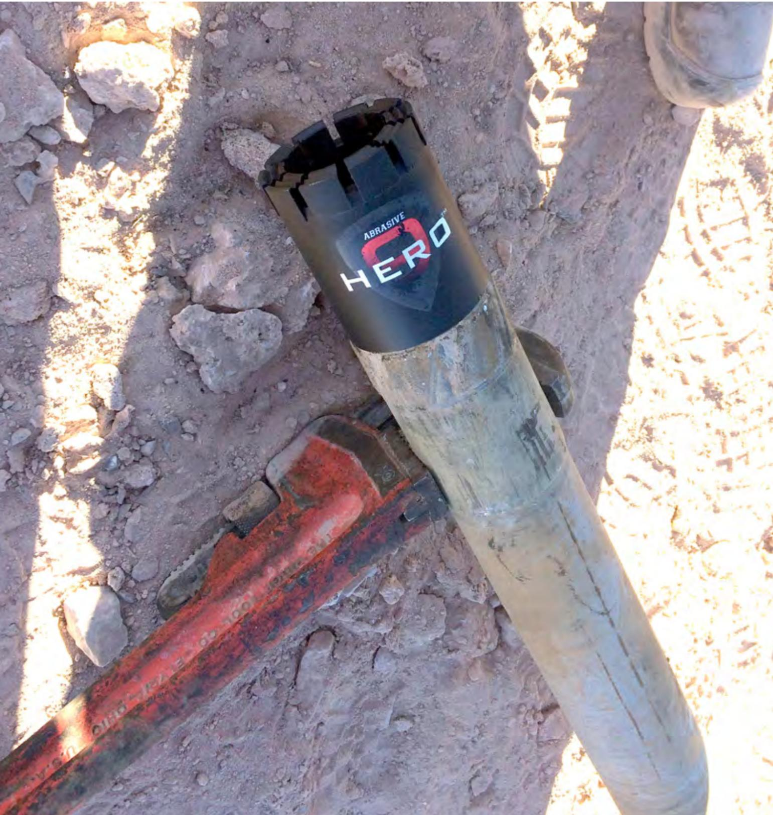
Getting the longest life possible for your core matrix is an important consideration if you want to run a productive and profitable drilling operation. Changing a drill bit takes time especially the farther down the hole it is, and the time spent replacing a bit is not productive. It is time when you are not recovering core and core recovery is the goal of diamond drilling.
