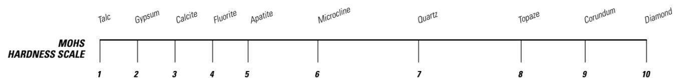
If you are using a pocket knife, the average hardness of this tool is approximately 6.0 to 6.5 and if you are using a metal saw, it should be around 6.5 to 7.0 on Mohs scale. For more details on how to perform a scratch test, or to order a Fordia etcher kit, contact your sales representative.
