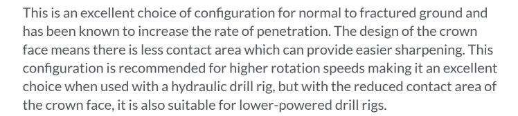
If you are using the Turbo Pie Shaped configuration and find that it isn't cutting well, you should consider switching the matrix. More often than not, the choice of matrix is not suitable for the ground conditions and may be the cause of poor cutting ability.
