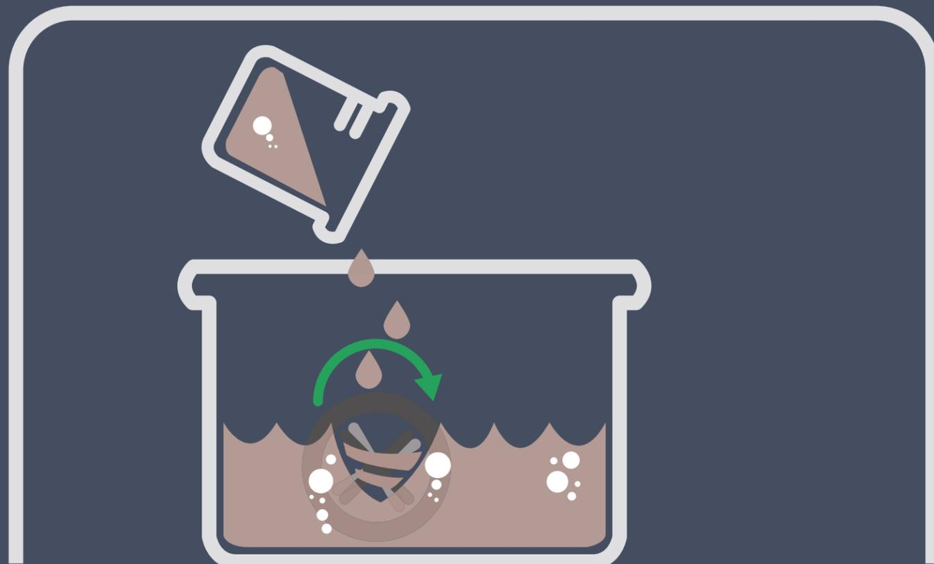
The mixing time will vary according to the temperature of the water. Colder water requires a longer mixing time.
