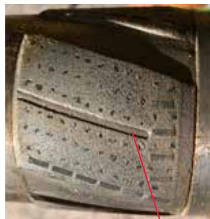
Wear indicator – no gauge checks
